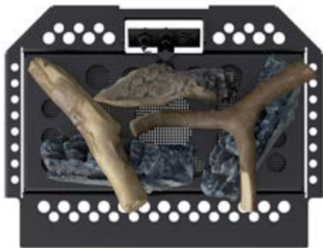
Fig. 20. Correct arrangement of decorative logs
