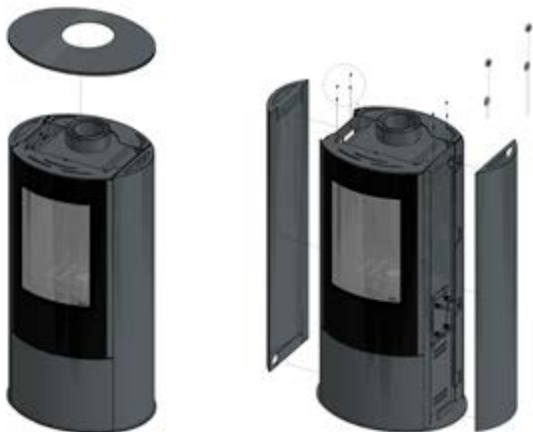
Figure 8. Removal of the top plate and the side panels
