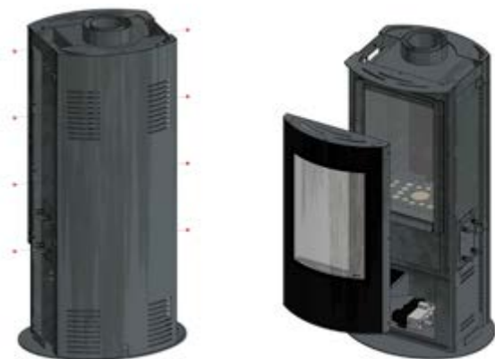
Figure. 10. Removal of the doors
